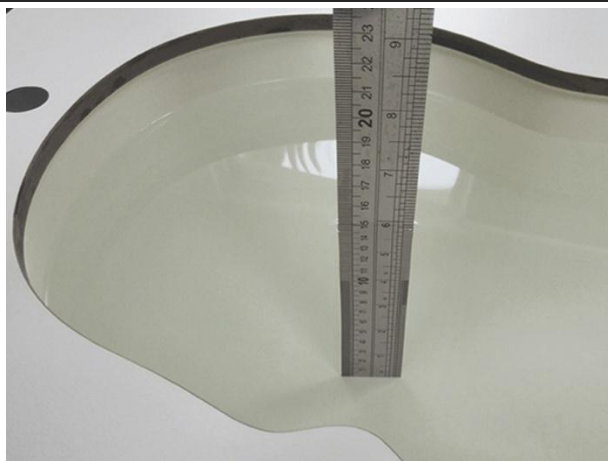
Liquid depth in the head phantom (2450MHz)
