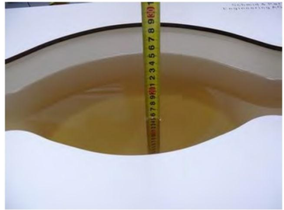
Liquid depth in the body phantom (835MHz)
