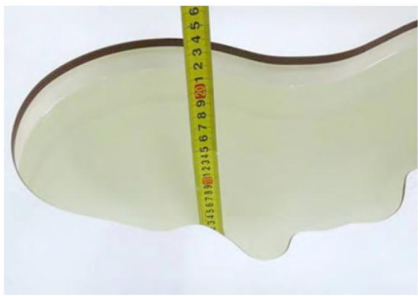
Liquid depth in the head phantom (1900MHz)
