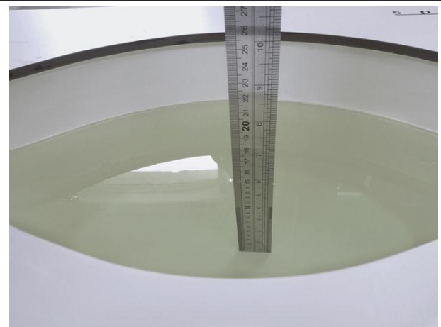
Liquid depth in the body phantom (2450MHz)
