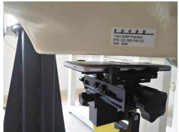
Body-worn Rear Side (10mm)
