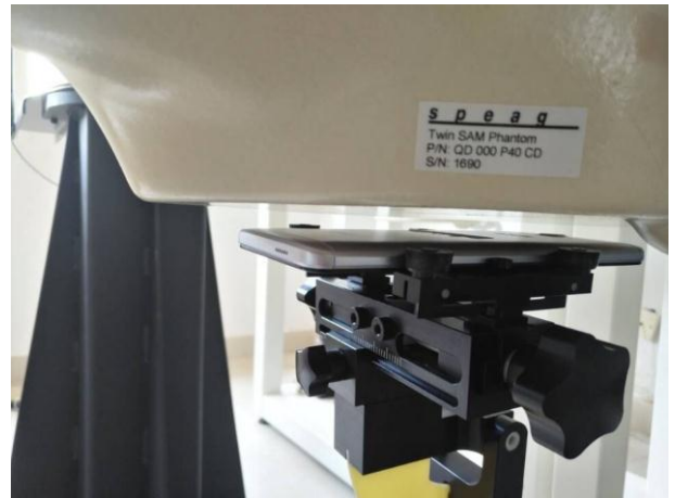
Hotspot mode - Rear Side (10mm)
