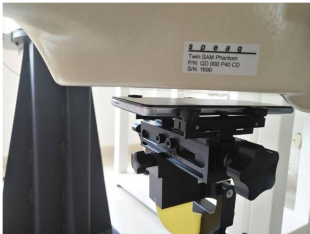
Body-worn Front Side (10mm)
