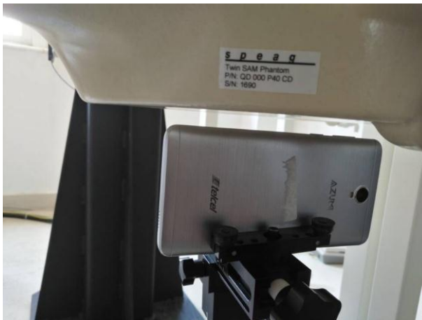
Hotspot mode - Right Side (10mm)
