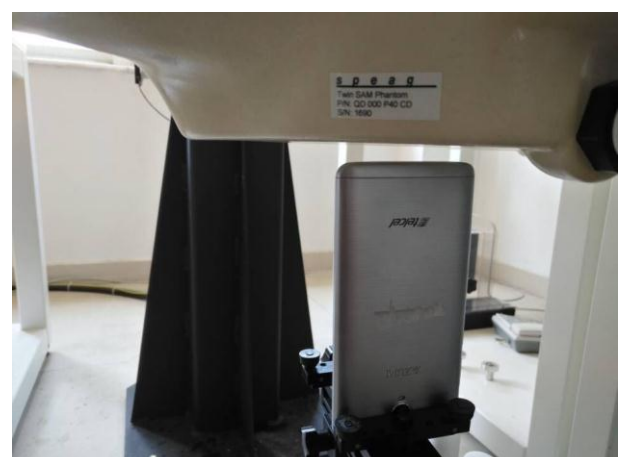
Hotspot mode - Bottom Side (10mm)
