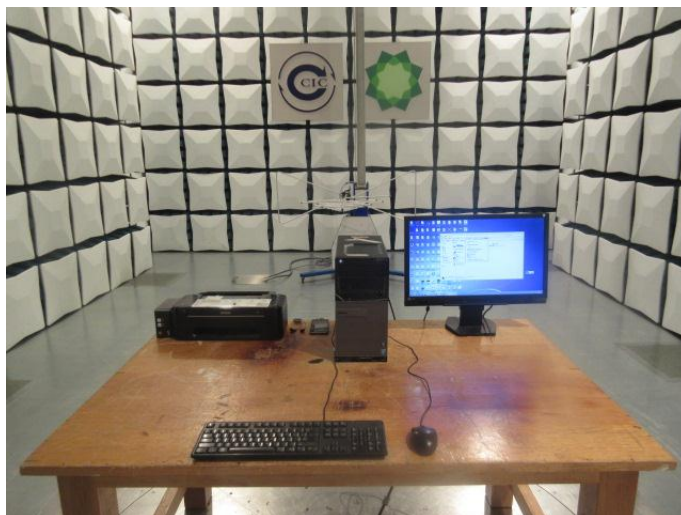
Radiated Emission (above 1GHz) Connect to PC
