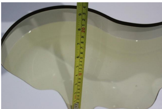
Liquid depth in the head phantom (2600MHz)
