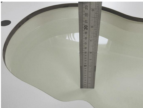
Liquid depth in the head phantom (2450MHz)
