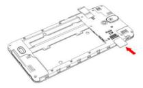
SIM card and the metallic contacts are facing the correct direction. Slide the SIM card into the slot until it doesn't move up any further.
