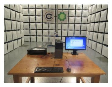
Radiated Emission (above 1GHz) Connect to PC
