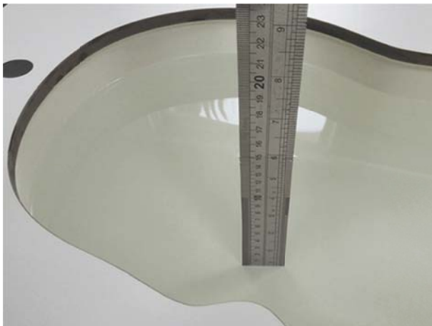
Liquid depth in the head phantom (2450MHz)
