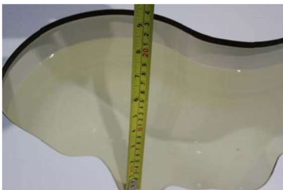
Liquid depth in the head phantom (2600MHz)
