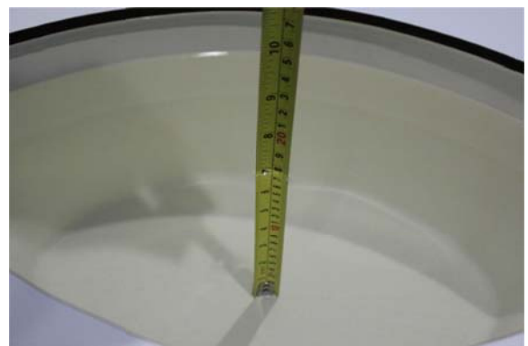
Liquid depth in the body phantom (2600MHz)
