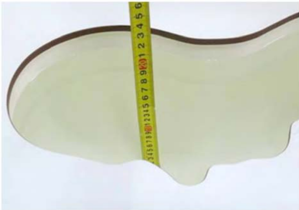
Liquid depth in the head phantom (835MHz)
