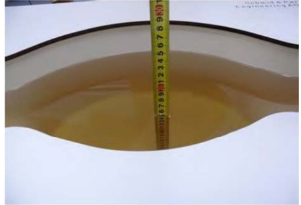
Liquid depth in the body phantom (835MHz)
