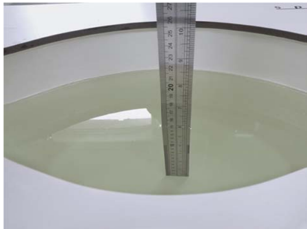
Liquid depth in the body phantom (2450MHz)
