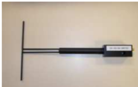
Figure 1 – Satimo COMOSAR Validation Dipole
