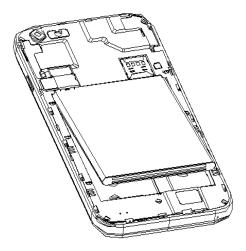
3. Insert the Micro-SIM card and SD card correctly .
