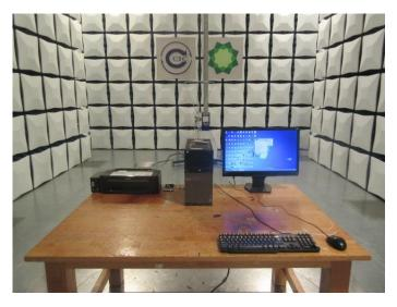
Radiated Emission (above 1GHz) Connect to PC
