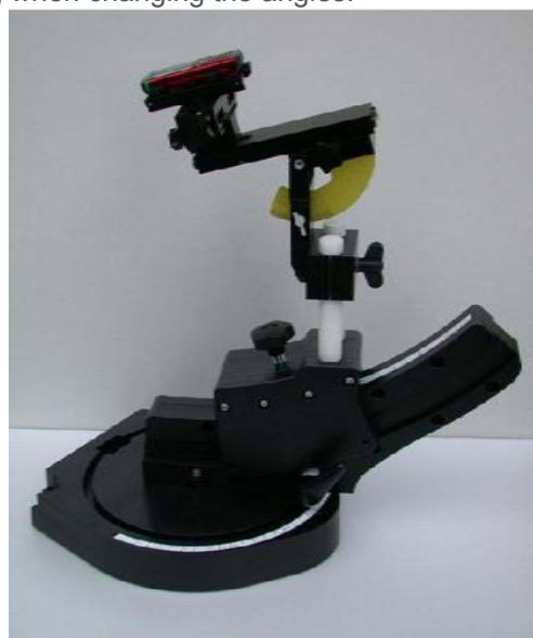
Device holder supplied by SPEAG
