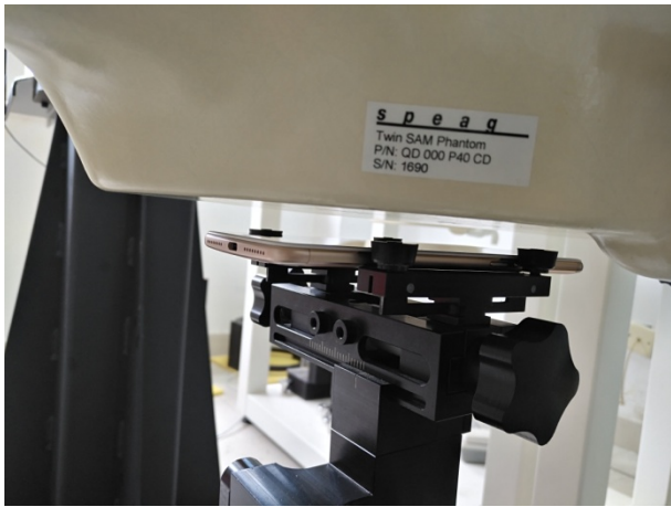
Body-worn Front Side (10mm)
