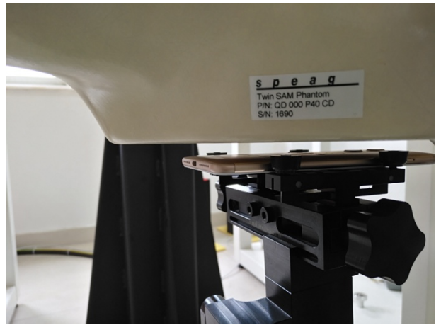
Body-worn Rear Side (10mm)
