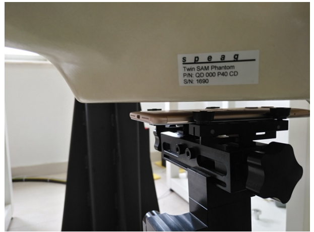
Hotspot mode - Rear Side (10mm)
