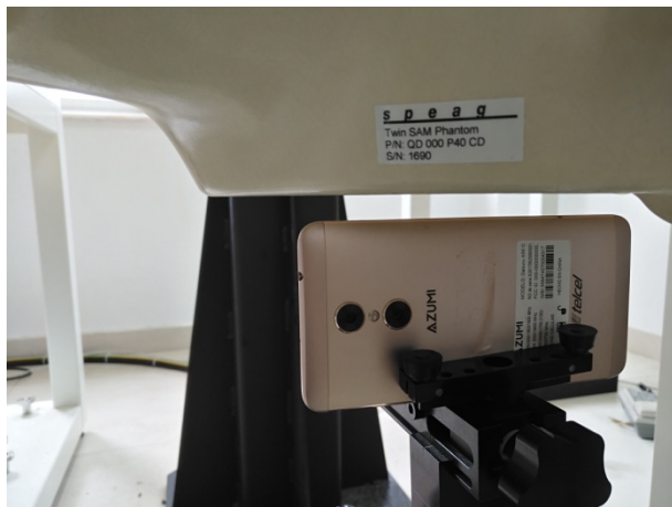
Hotspot mode - Left Side (10mm)
