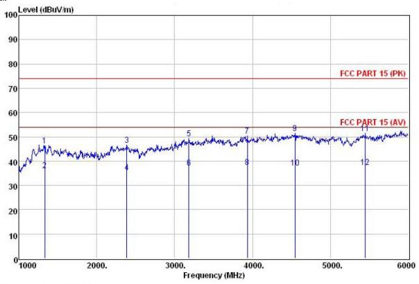
: 3m chamber : FCC PART 15 (PK) 3m BBHA9120(>1GHZ) VERTICAL : 205RF Site Condition
