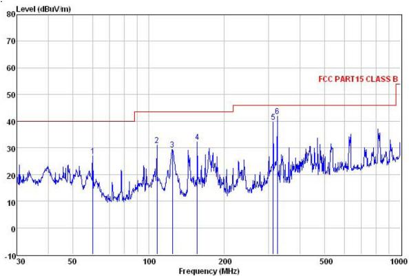
: 3m chamber : FCC PART15 CLASS B 3m VULB9163(2012.4.1) VERTICAL : 205RF Condition
