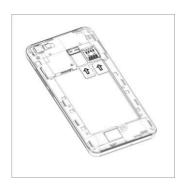
Please insert the SIM card according to the label on the phone. Make sure that the clipped corner of the SIM card and the metallic contacts are facing the correct direction. Slide the SIM card into the slot until it doesn't move up any further.
