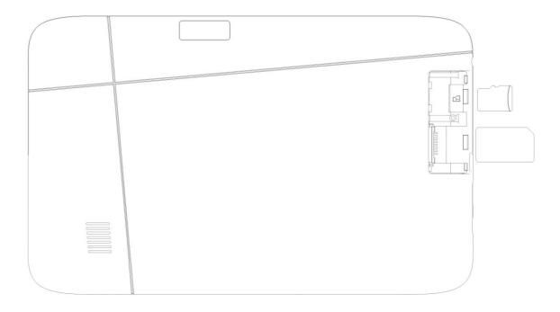
Insert the SIM or USIM card when you need a cellular service. Do not insert a memory card into the SIM card slot.
