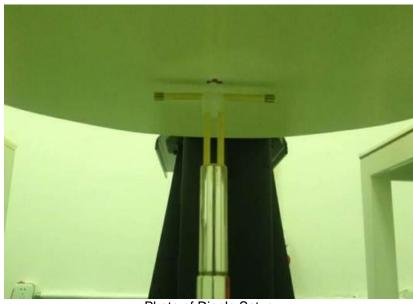
Photo of Dipole Setup
