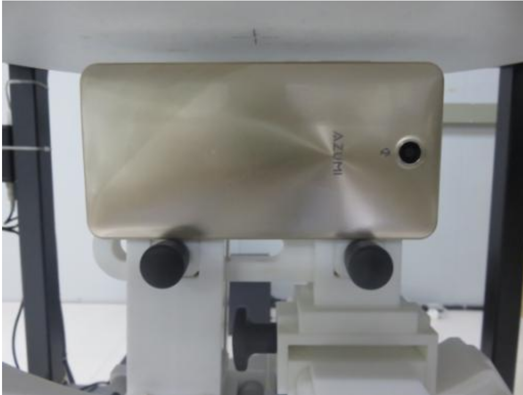
10mm body-worn Right Side Setup Photo(hotspot)
