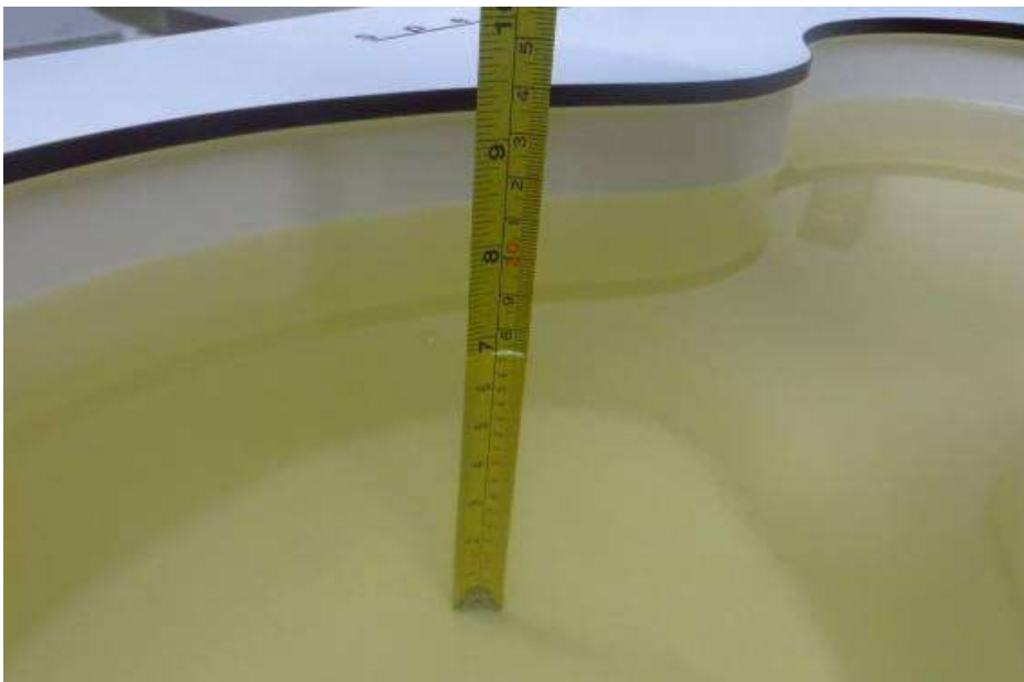
Liquid depth in the Body Phantom (1900 MHz) (depth>15cm)
