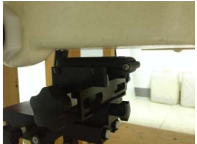
Back of the EUT with 1 cm Gap
