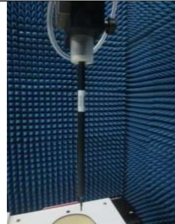
Fig. 8.2 Photo of E-Field Probe
