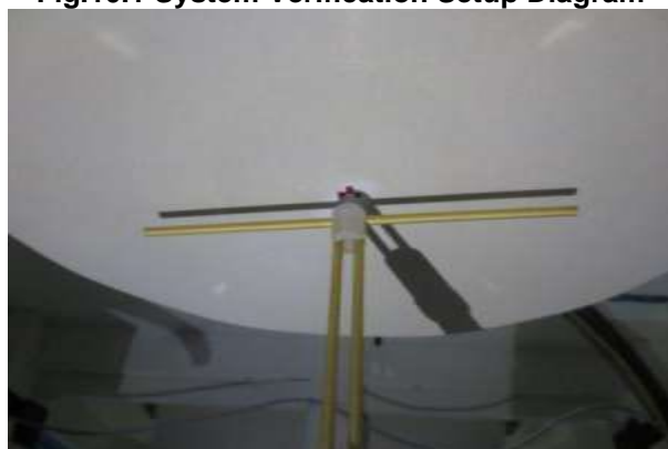
Fig.10.2 Photo of Dipole setup
