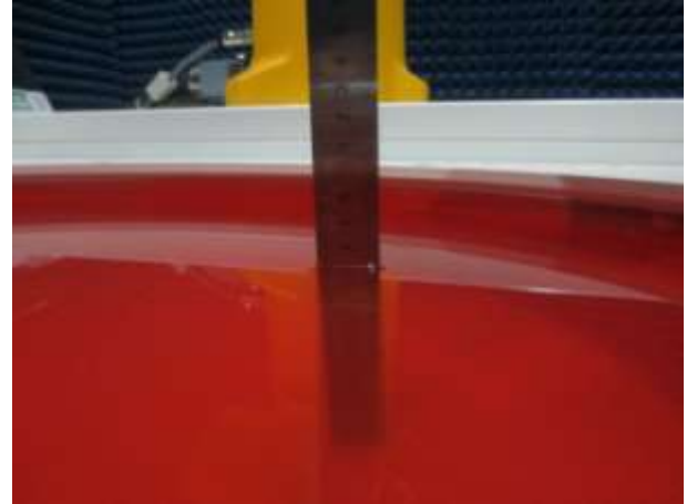
Fig. 9.2 Photo of Liquid Height for Body SAR of (700MHz~1000MHz) (depth>15cm)
