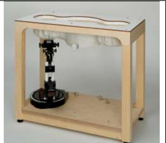
Fig. 8.7 Photo of SAM Twin Phantom
