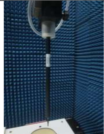
Fig. 8.2 Photo of E-Field Probe
