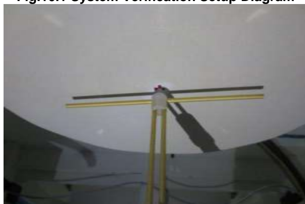
Fig.10.2 Photo of Dipole setup
