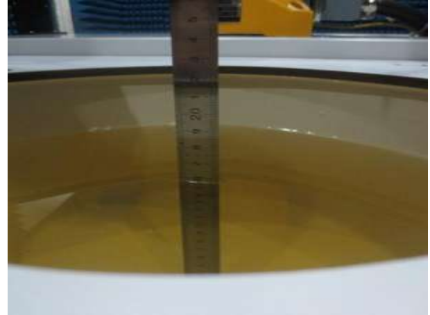
Fig. 9.2 Photo of Liquid Height for Body SAR
