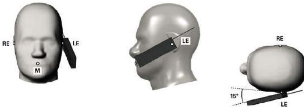
Fig.11.4 Illustration for Tilted Position
