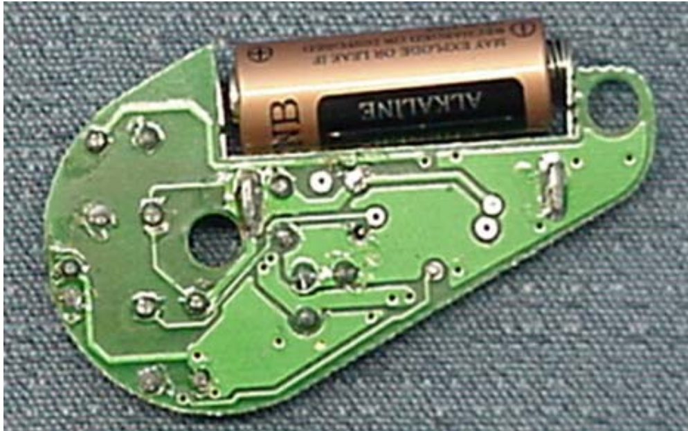
Transmitter internal view
