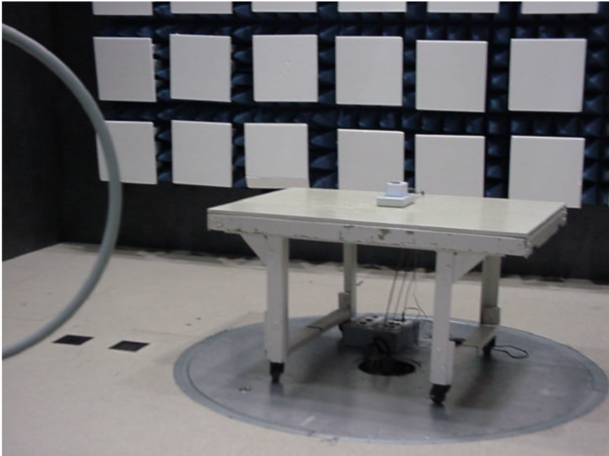
Figure 13 - Radiated Emissions Test Setup, prescans (9KHz to 30 MHz)
