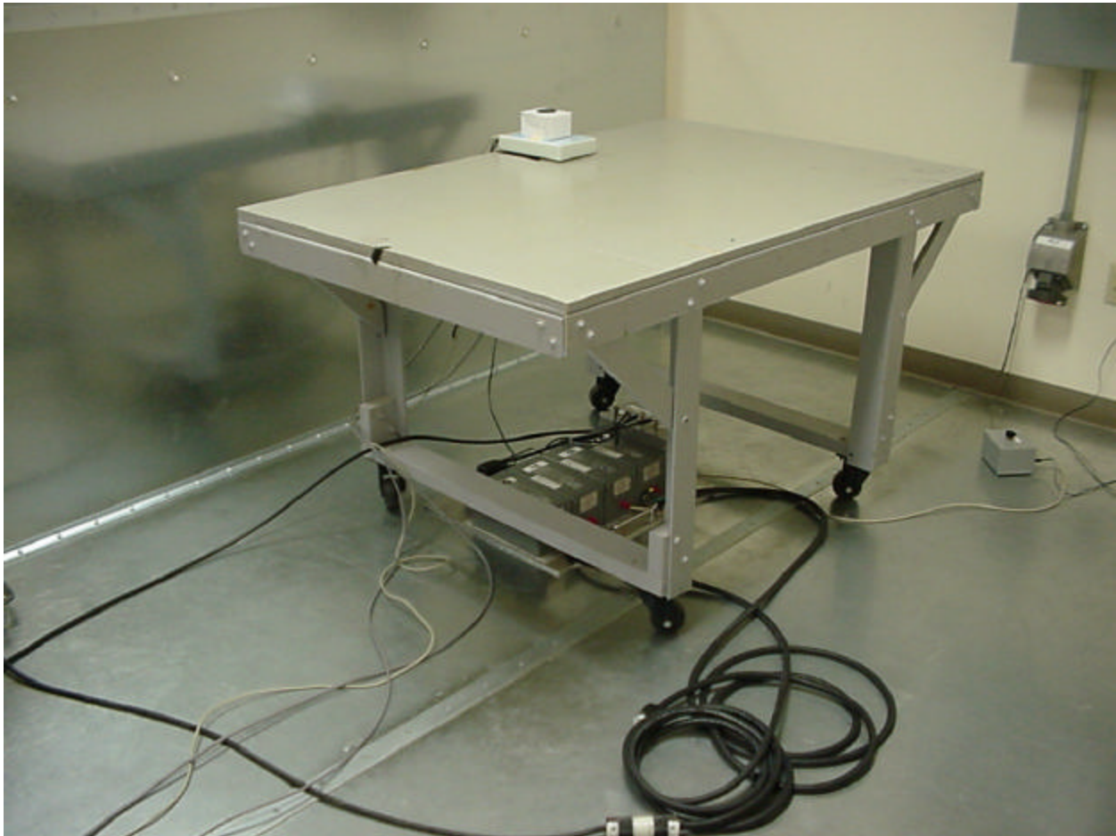
Figure 19 - Conducted Emissions Test Setup (Front) CUI Stack Model DSA-0151A-12
