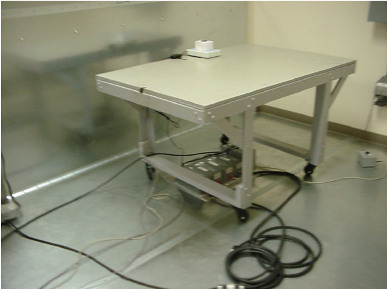
Figure 17 - Conducted Emissions Test Setup (Front) CUI Stack EPA-121DA-12
