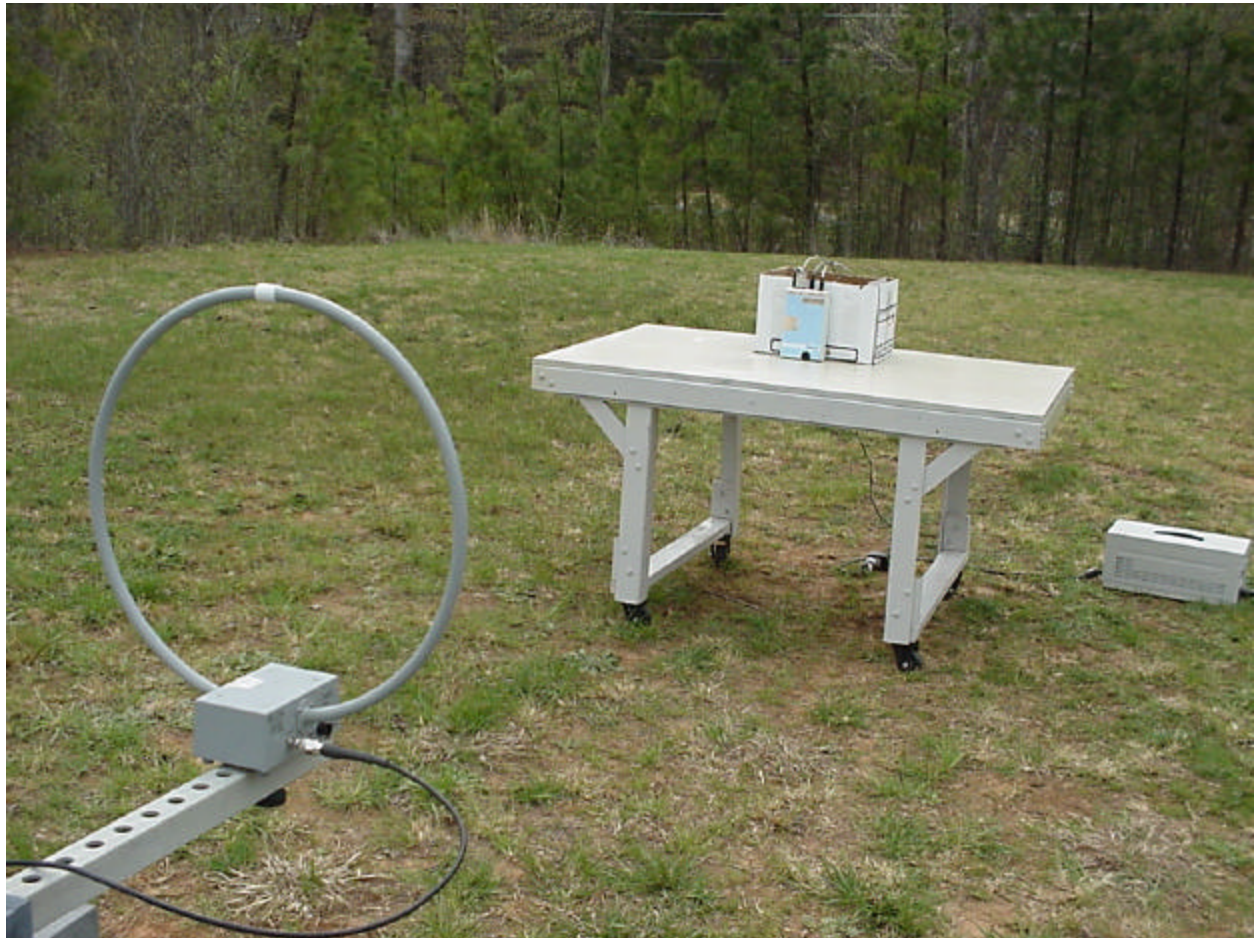
Figure 14 - Radiated Emissions Test Setup (9KHz to 30 MHz)
