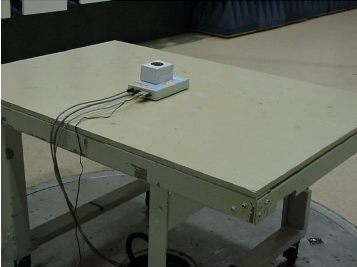
Figure 12 - Radiated Emissions Test Setup (Chamber - Back)
