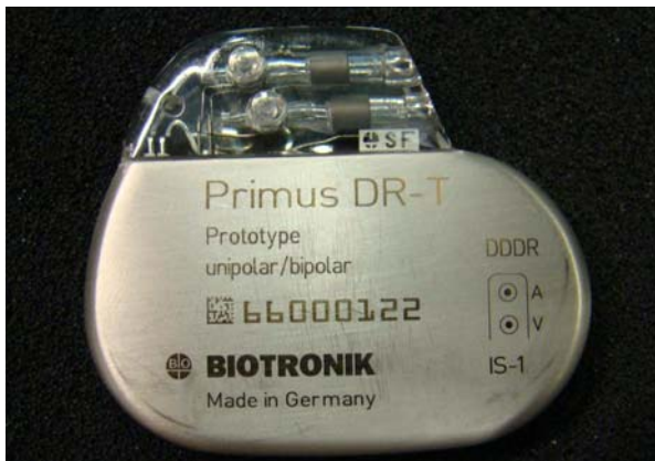
Figure 7.1.1 Front view of the Primus Pacemaker.
