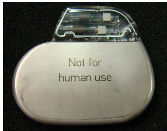
Figure 7.1.2 Rear view of the Primus pacemaker.
