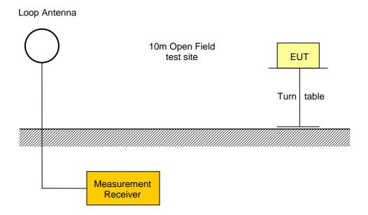
The eut is placed on a non-metallic table. Any emission is received by a loop antenna and measured via a measurement receiver connected to the loop antenna. To obtain the maximum emission the eut is rortated through 360°.
