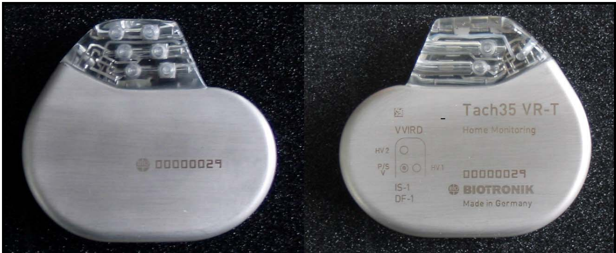
Figure 7.1.1 Photograph of a Tach 35 Implantable Cardioverter Defibrillator (ICD).
