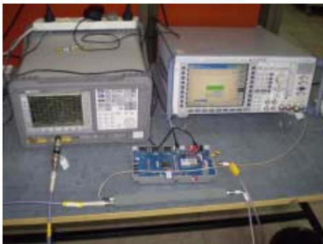
Photograph 8.1.1 Peak output power test setup
