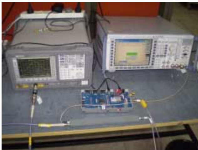
Photograph 7.3.2 Spurious emission test setup
