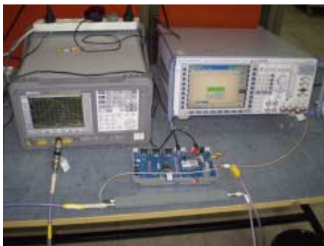
Photograph 8.2.2 Occupied bandwidth test setup
