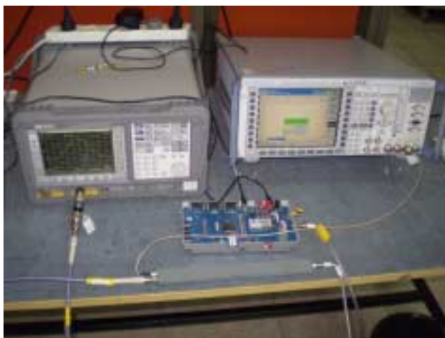
Photograph 7.1.2 Peak output power test setup
