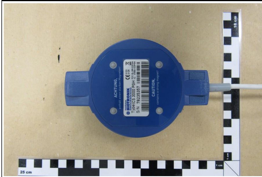
AE2: PGH 3000 programming head bottom
