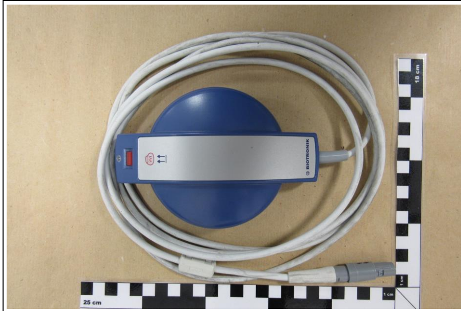
AE2: PGH 3000 programming head top
