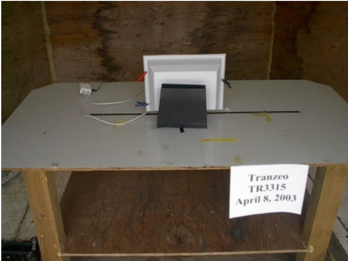
Front Emissions Test Setup
