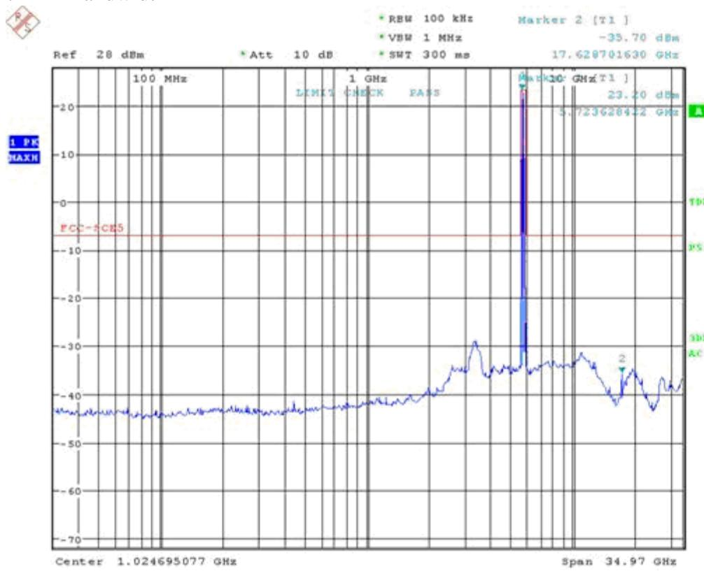
The above plot shows the worst case conducted output of the transmitter. It should be noted that the EUT is not transmitting on two channels simultaneously. All conducted harmonics are at least 30 dBc.
