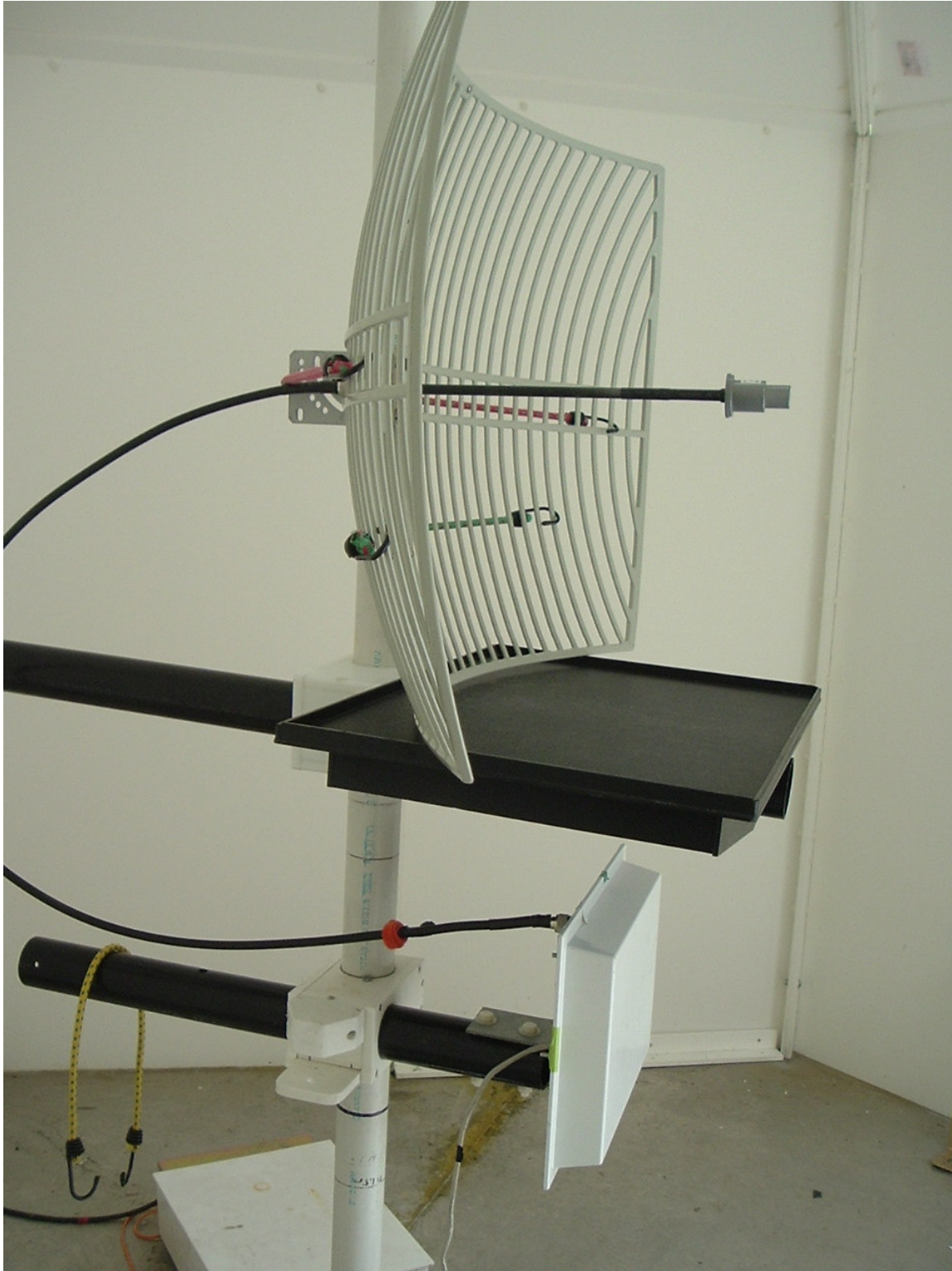
Grid antenna(26 dBi)
