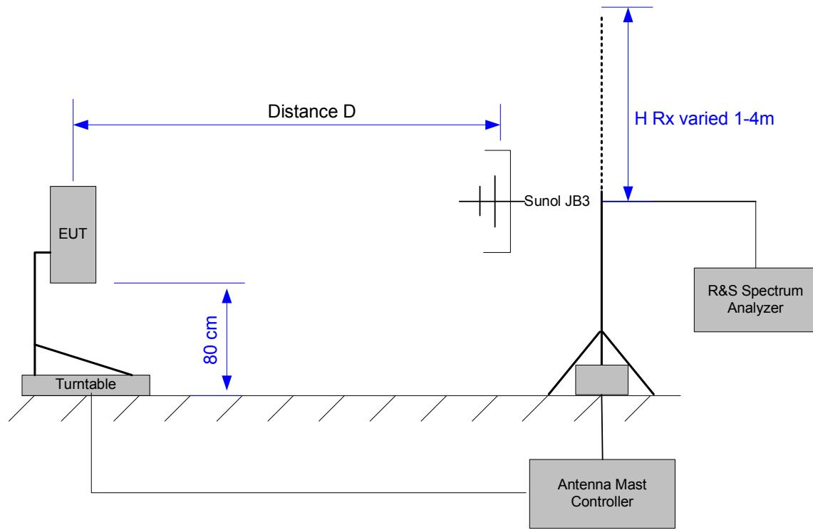
Note: Measurements below 1 GHz were performed with the Sunol JB3 antenna with a measurement distance of 3 m. Compliance above 1 GHz is covered in Section 5.0.
