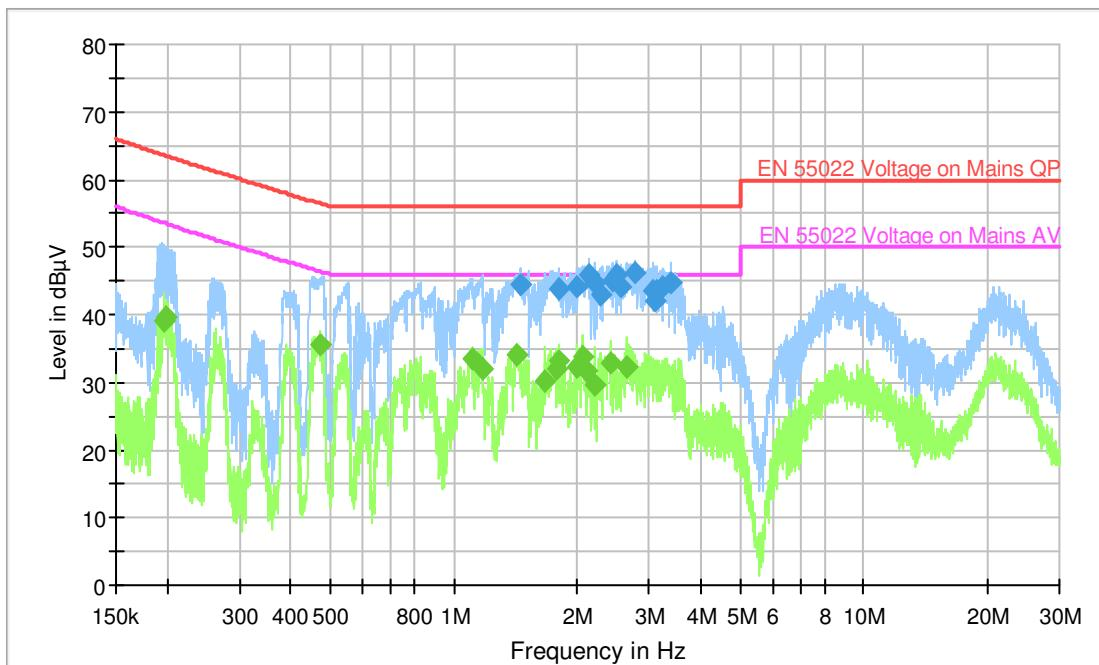
The blue measured curve represents the quasi-peak measurement. The green measured curve represents average values. The measured points marked with squares.
