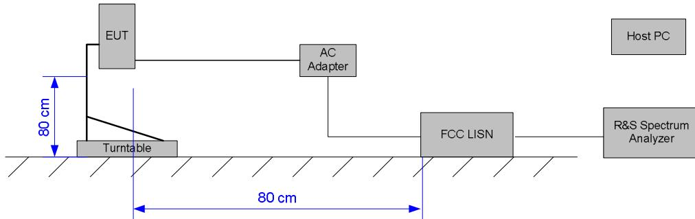
*Note: The unused LISN terminal is terminated with a 50 ohms terminator.*
