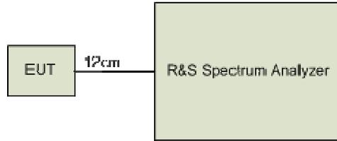
6.3.2 Test Setup Block Diagram – Radiated Measurements
