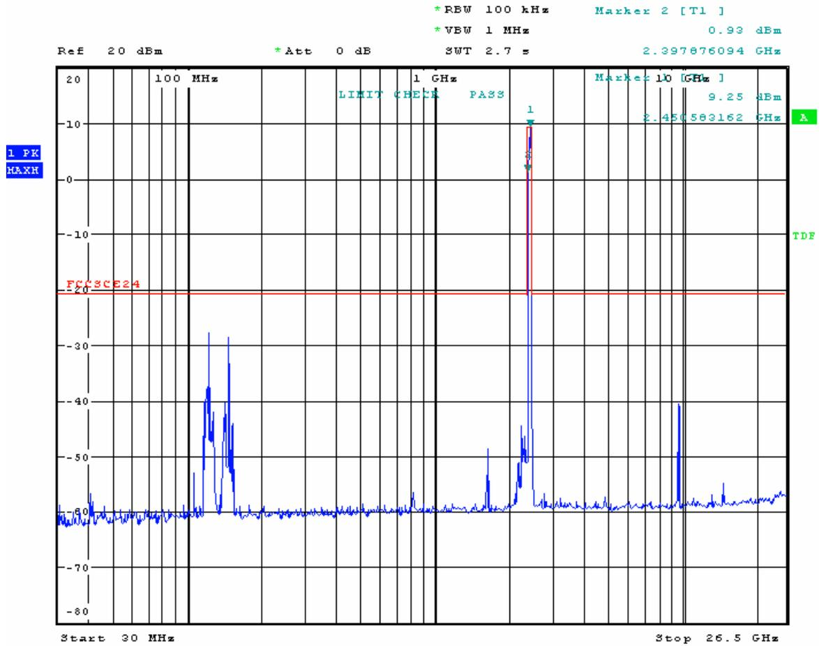
The above plot shows the conducted output of the transmitter. There are no conducted harmonics within the 30 dBc limit.
