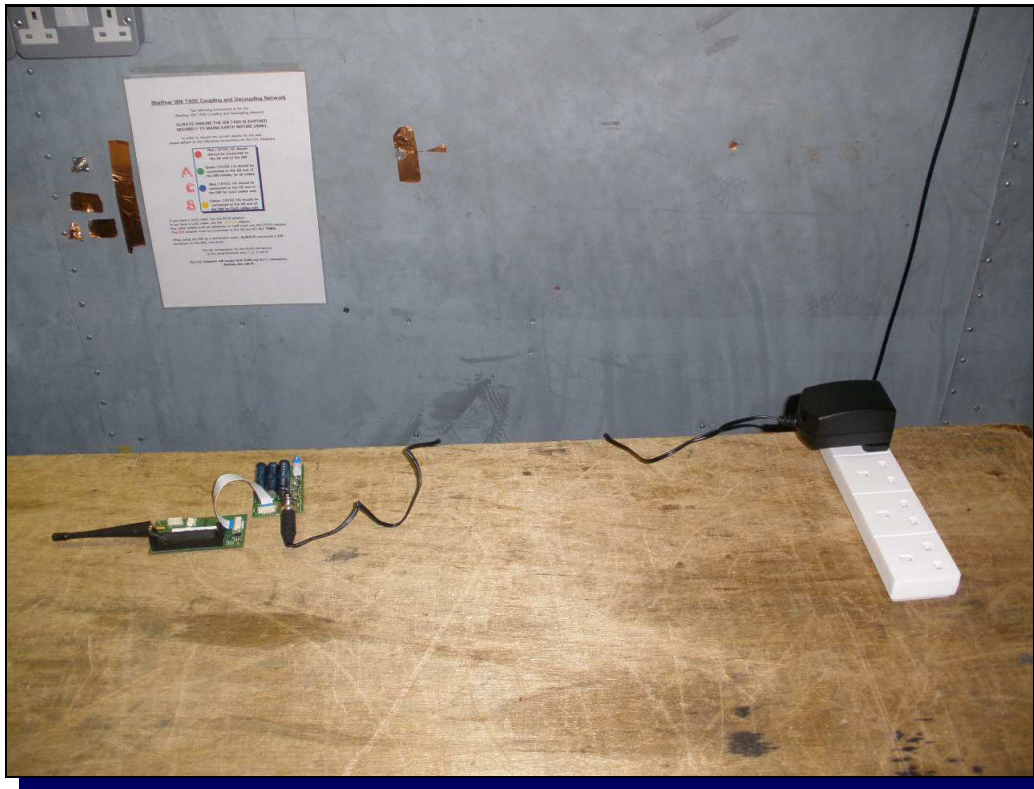
Photograph 1 Conducted Emissions - Front
