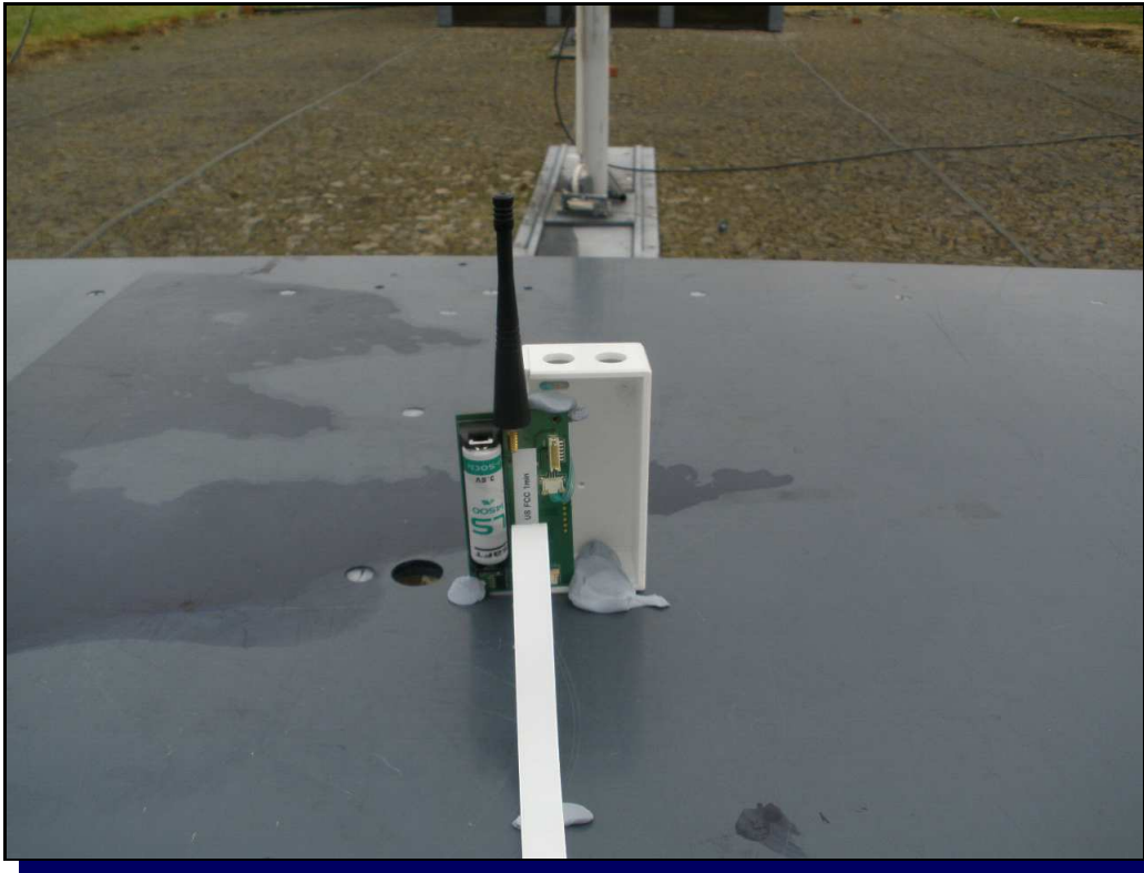
Photograph 5 Radiated Emissions - Upright, Close-up
