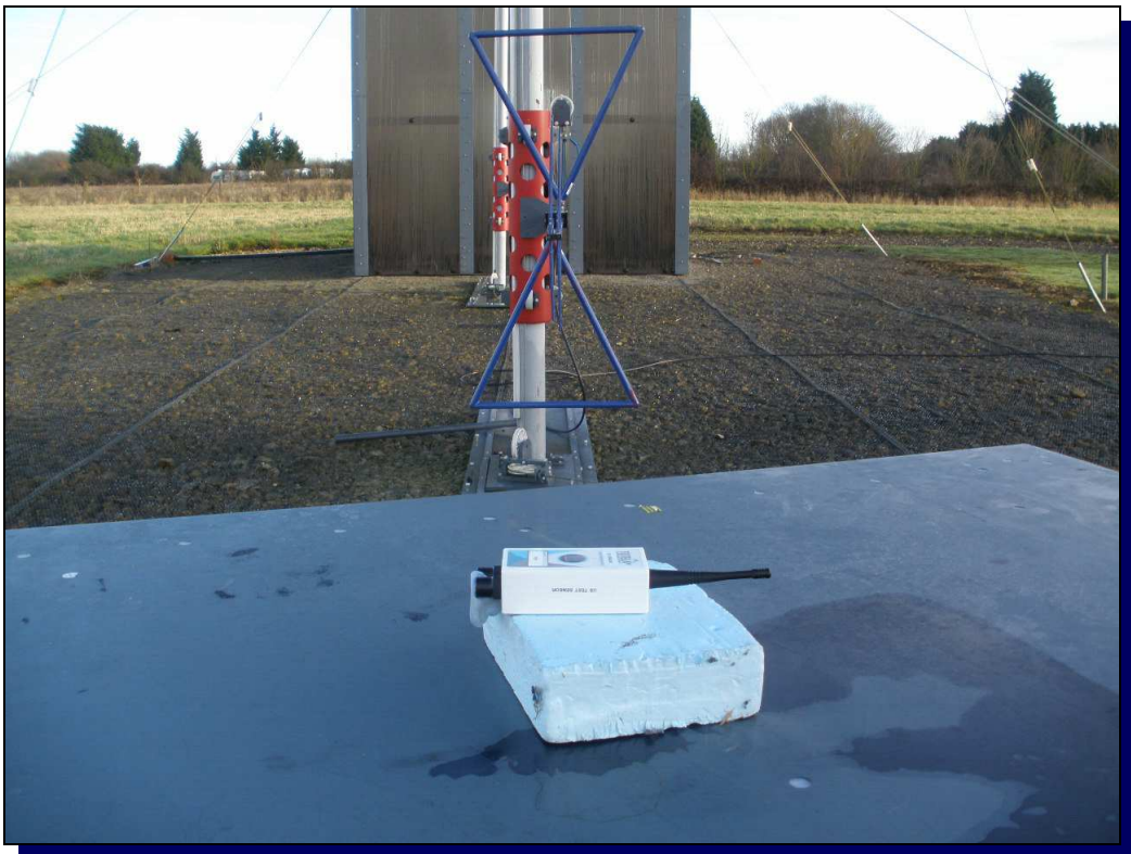
Photograph 16 Radiated Emissions - Data Transceiver - Flat
