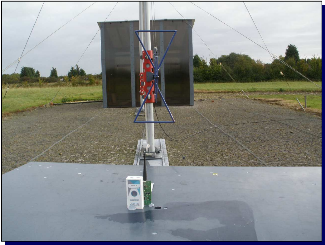
Photograph 3 Radiated Emissions - Upright, Front
