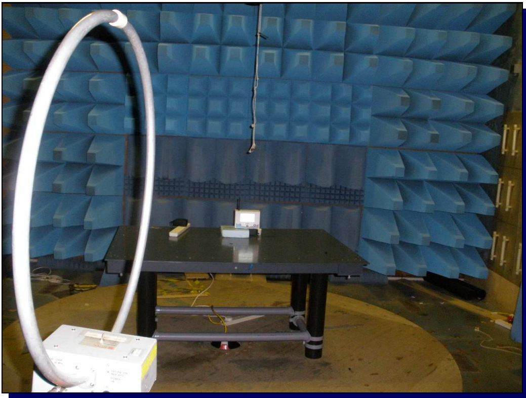
Photograph 19 Radiated Emissions - Below 30MHz - Controller
