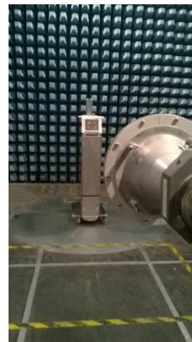
PHOTO N°3 SETUP FOR RADIATED MEASUREMENT >1GHz
