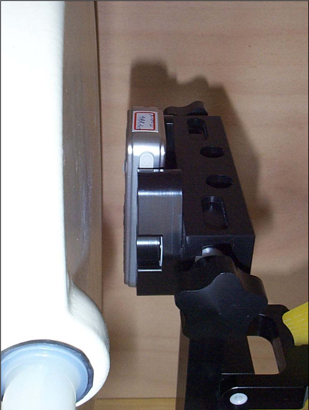
Spacing from flat phantom was adjusted at 1.5 cm.
