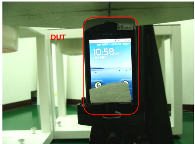
Top Side of the DUT with Phantom 1 cm Gap (DUT without Earphone)
