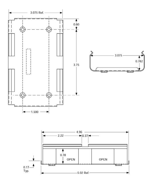
Figure 2- Snap-in Mounting Bracket
