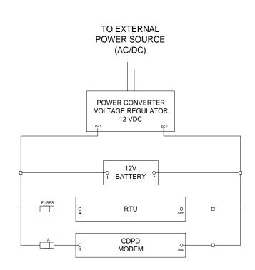
**Figure 6 - Power Connections**
