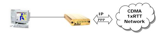
If the host establishes a PPP link to the AirLink modem, a second PPP link is created between the modem and the host. IP packets can then be sent to and received from the 1xRTT network.
