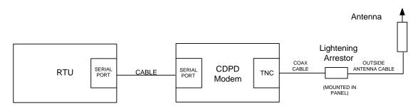
Figure 5 - RTU to Raven setup
