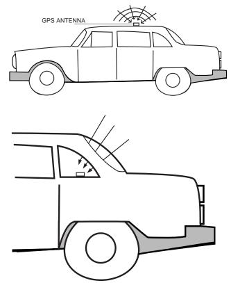
Figure 2 – Optimum GPS antenna positioning on a vehicle.
