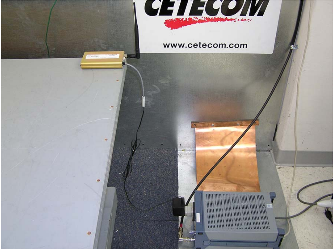
Test setup – AC Line Conducted Emissions Raven
