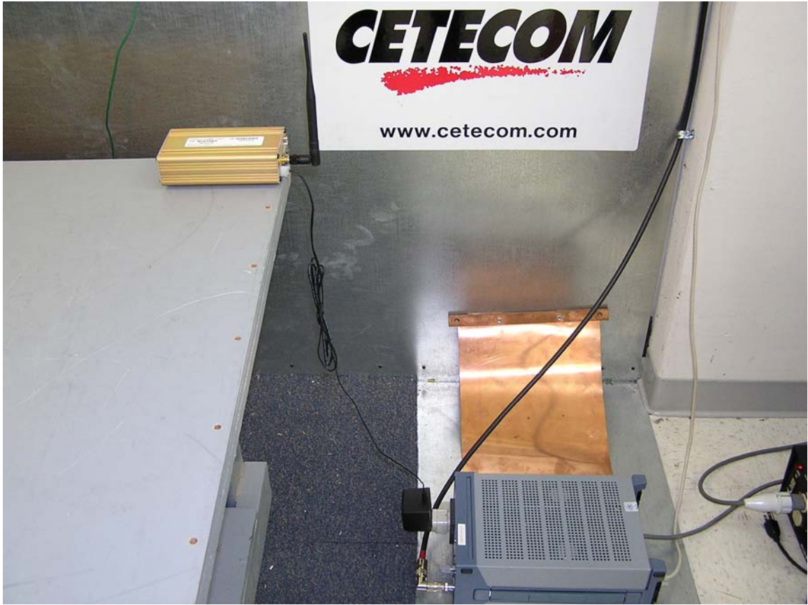
Test setup – AC Line Conducted Emissions Pinpoint
