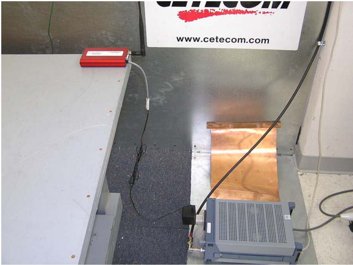
Test setup – AC Line Conducted Emissions Redwing
