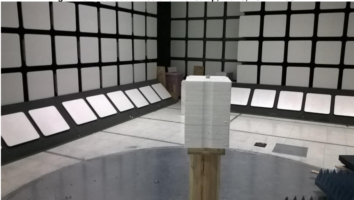
Figure 46 - Radiated Emissions Test Setup, Y-axis, 1GHz – 25GHz
