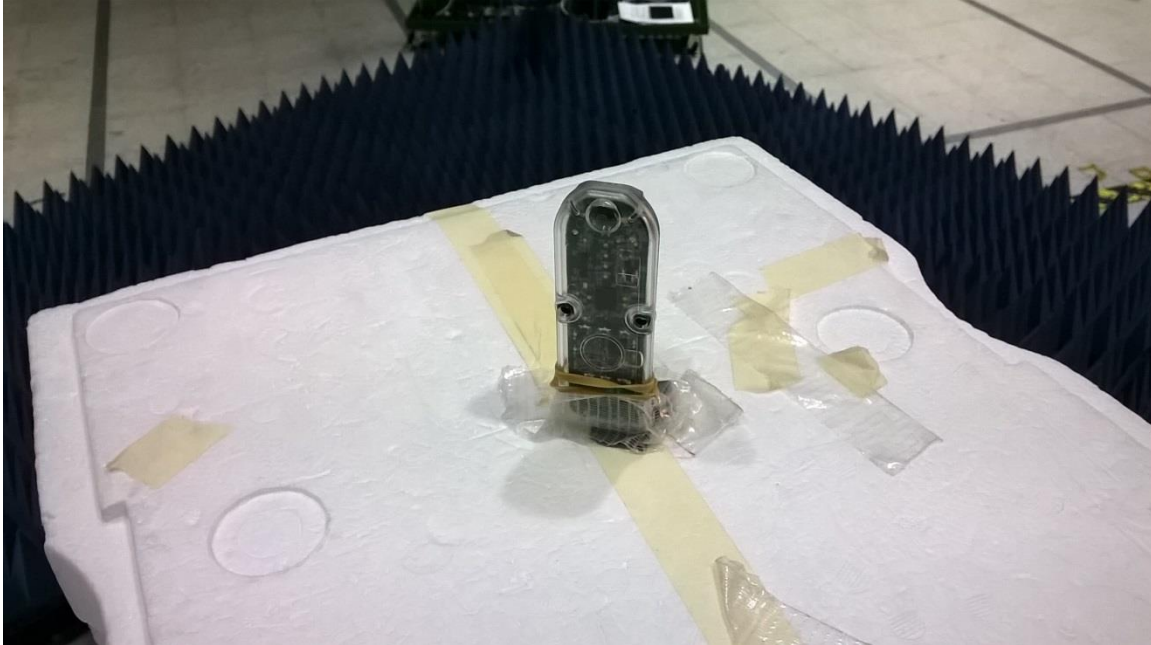
Figure 45 - Radiated Emissions Test Setup, X-axis, 1GHz – 25GHz
