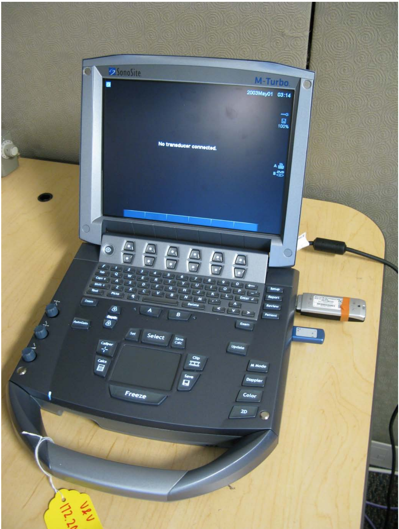
Illustration 1: M-Turbo unit with Bluetooth and 802.11 Dongles inserted
