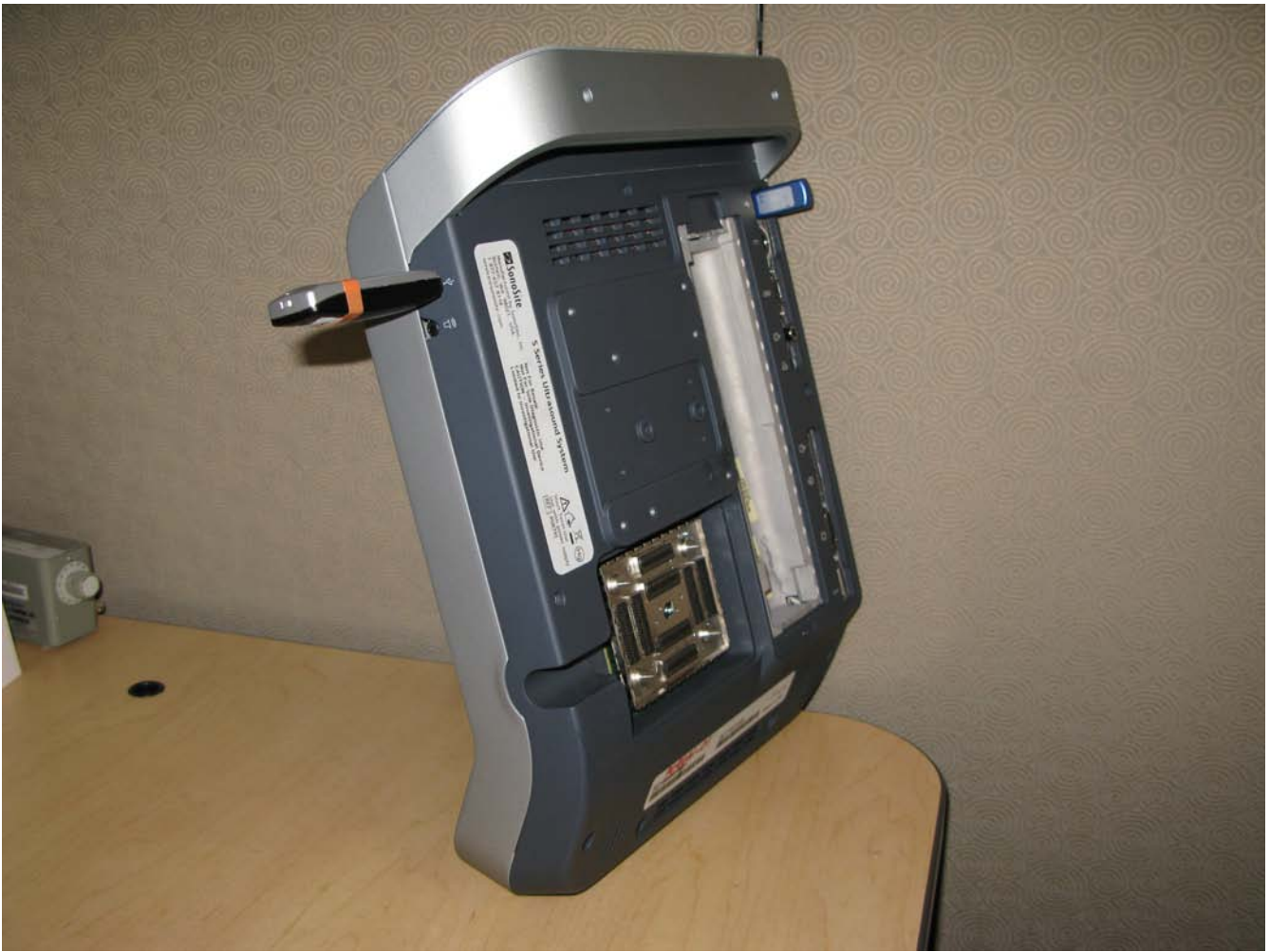
Illustration 2: Turbo S view from backside showing placement of Bluetooth and 802.11 dongles
