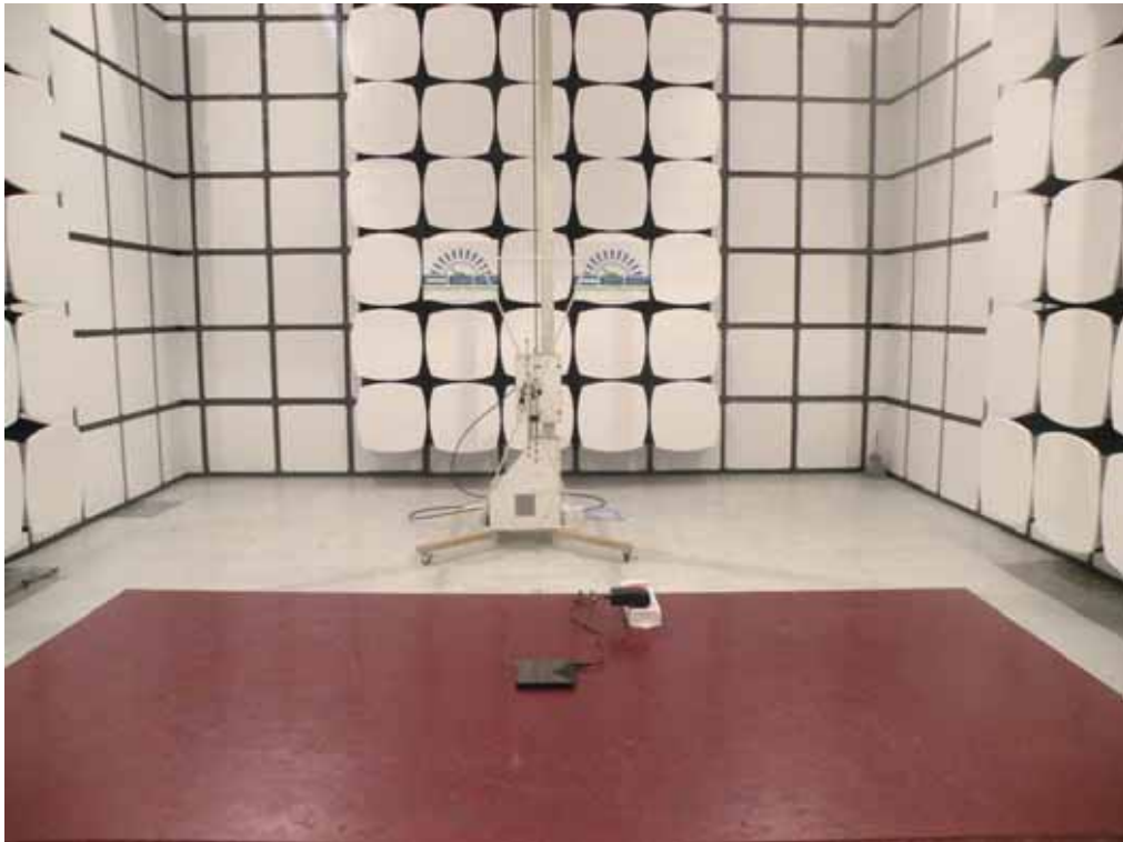
Radiated Emission Test Setup in Chamber
