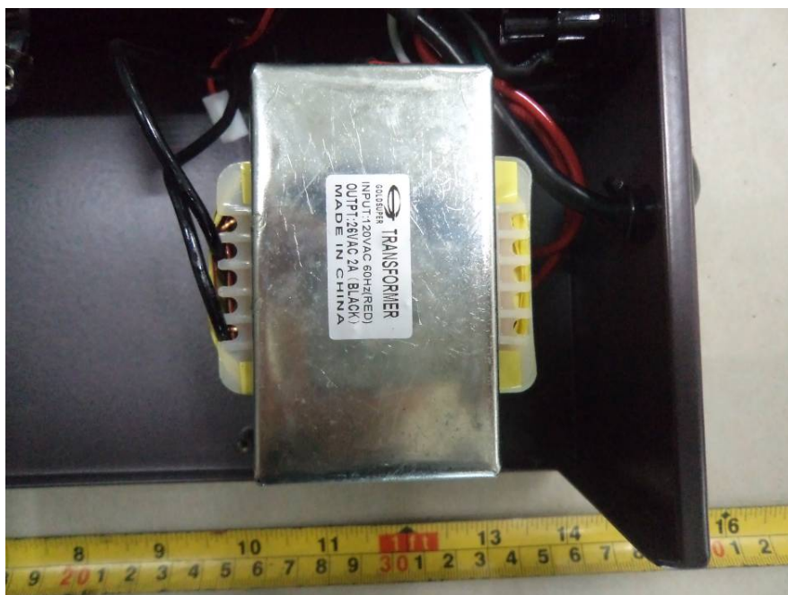
EUT –Transformer View (DC Power)
