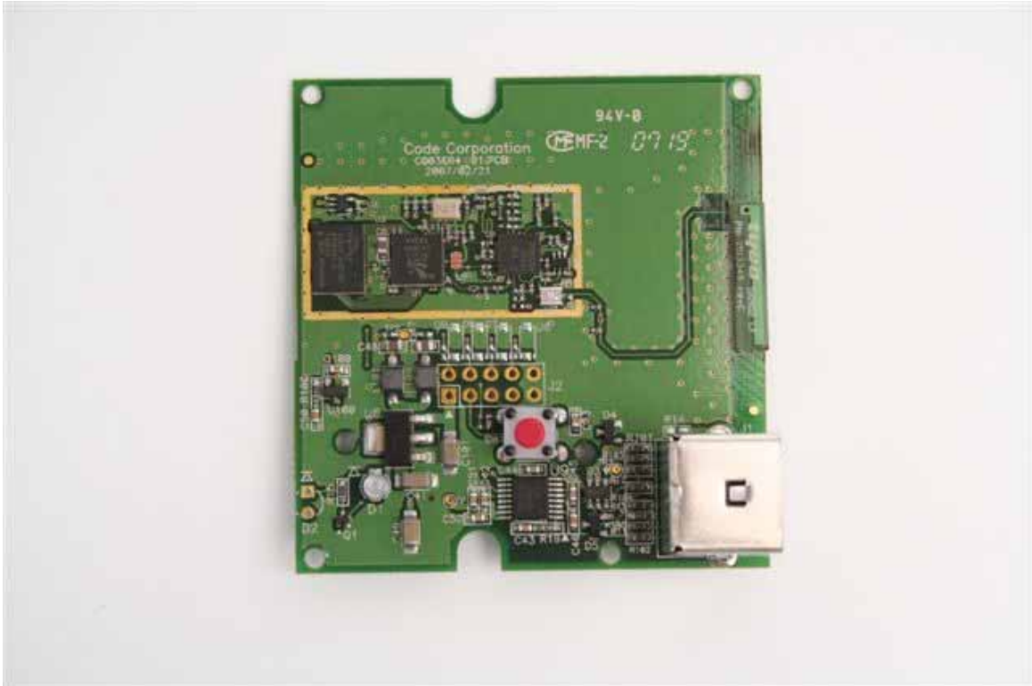
Photograph 7 - Top Side of PCB with RF Shield Removed
