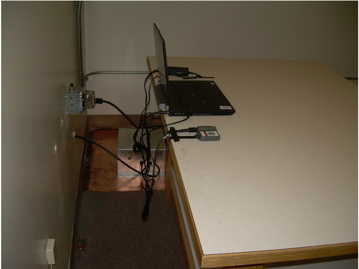
Back View Conducted Disturbance Worst Case Configuration
