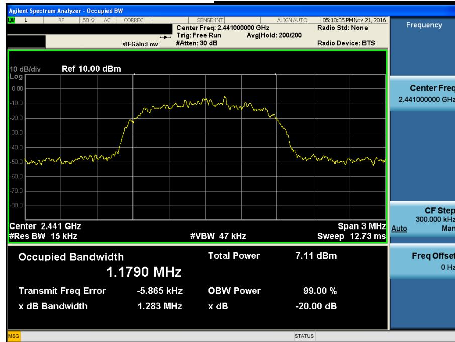
**20 dB Bandwidth****Highest Channel & Modulation : 8DPSK**
