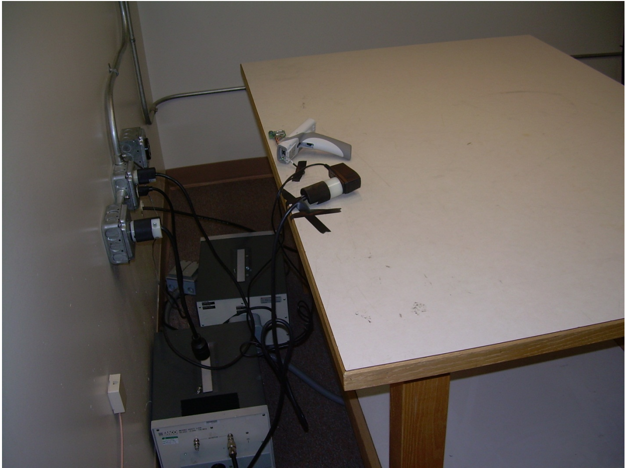
Back View Conducted Disturbance Worst Case Configuration
