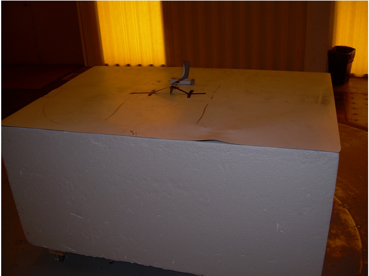
Front View Radiated Disturbance Worst Case Configuration – EUT on Edge
