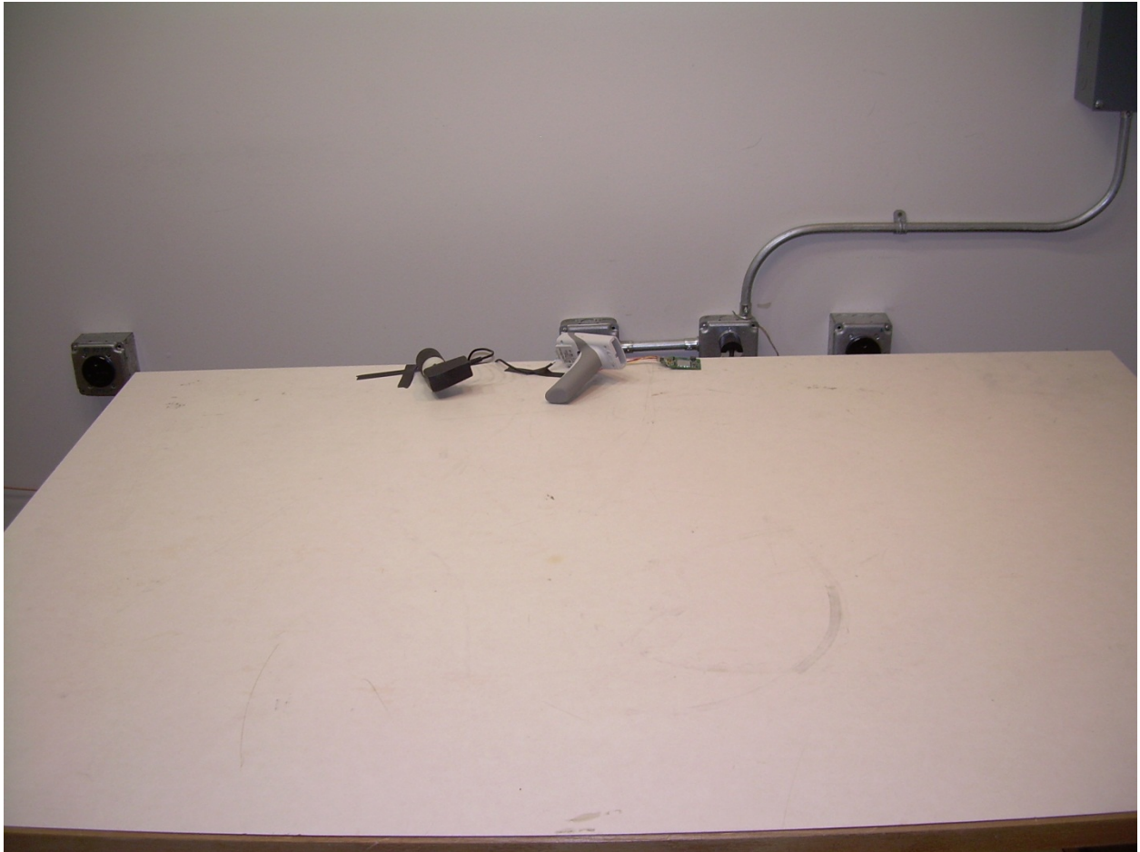
Front View Conducted Disturbance Worst Case Configuration
