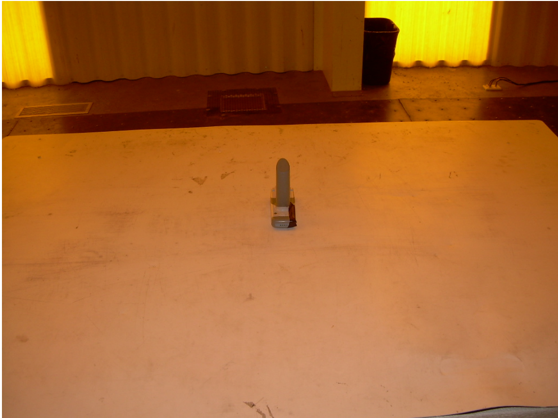
Photograph 3 – Front View CR2612_01 Radiated Emissions Setup – Horizontal Configuration
