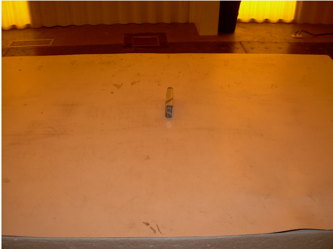
Photograph 5 – Front View CR2611_01 Radiated Emissions Setup – On Edge Configuration
