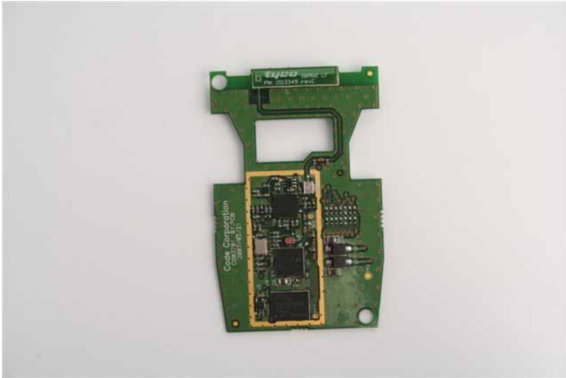
Component Side of PCB with RF Shield Removed
